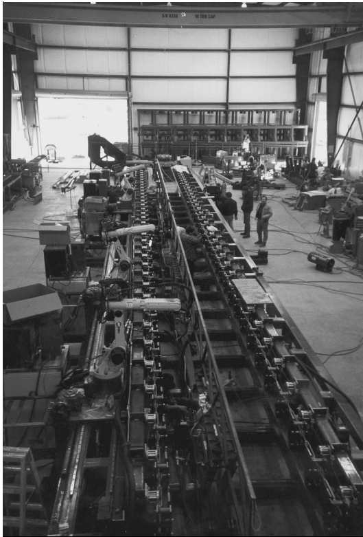
Plate 3 Multiple robot welding system
