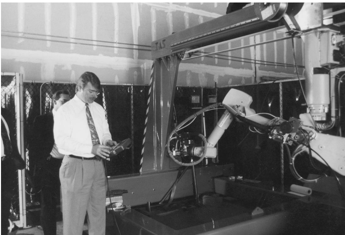
Plate 1 Robots mounted on overhead gantry
