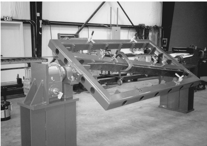
Plate 4 Positioning mechanisms allow rapid jiggging of complex components
